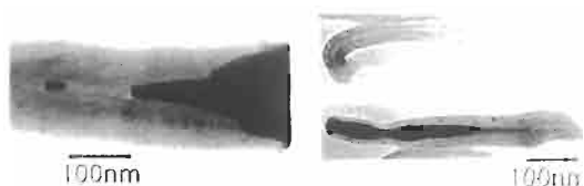
Fig. 3. TEM images of CNTs obtained by CVD of nickel phthalocyanine on a quartz substrate at 800°C: the bottom of the tube (right) and tip of the tube (left).
